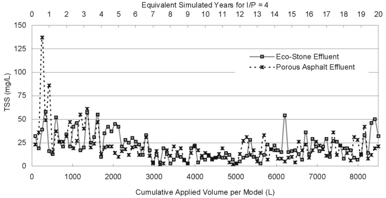
Fig. 8. Long-term effluent TSS for Eco-Stone and porous asphalt.
