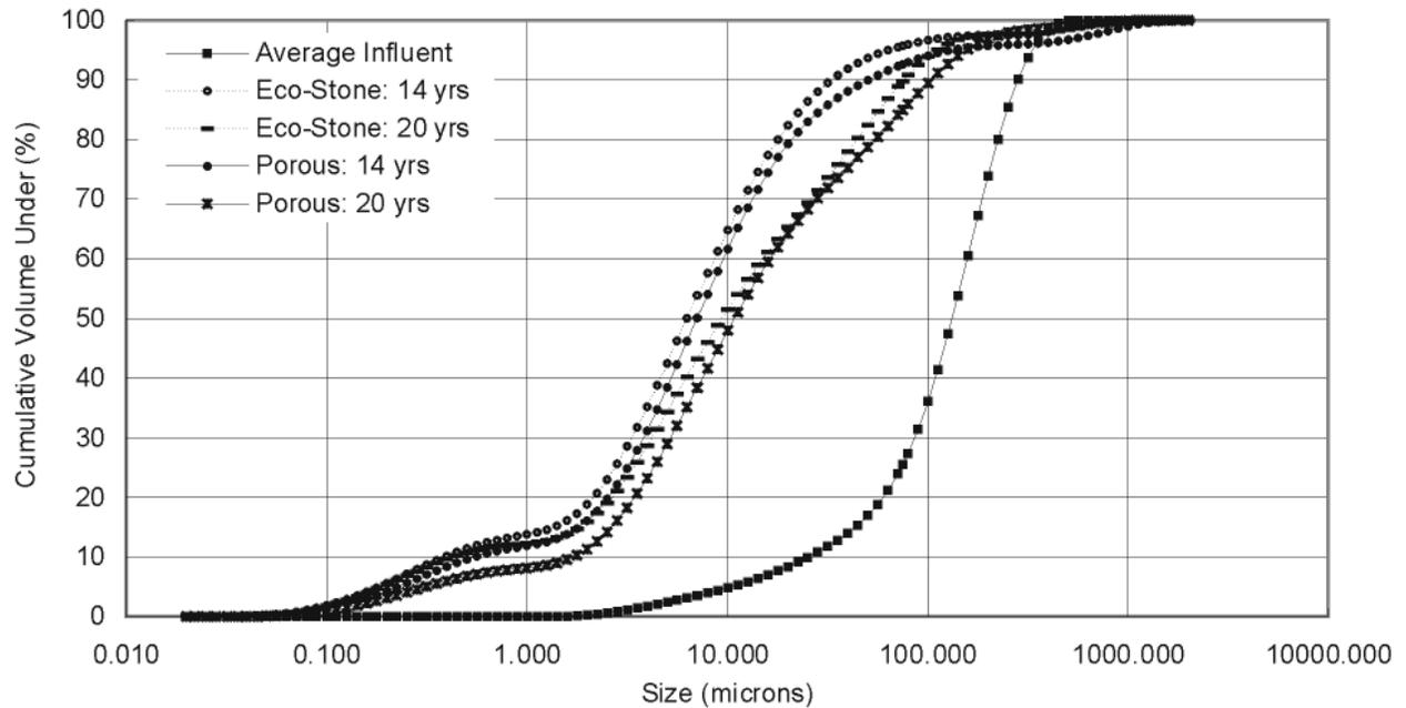
Fig. 9. Particle size distribution for the influent and effluent for long-term laboratory simulation for sub-250- $\mu\text{m}$  street sweepings.
