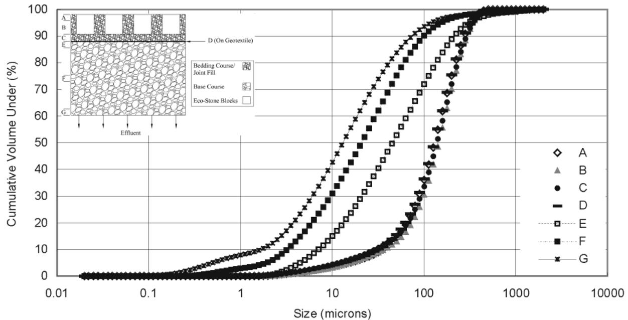
**Fig. 5.** Particle size distributions for Eco-Stone layers throughout pavement model after simulation of 20 years of runoff (layer locations shown upper left corner).
