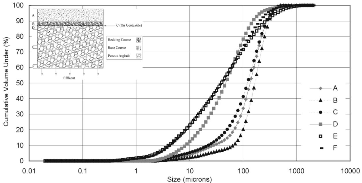
**Fig. 6.** Particle size distributions for porous asphalt layers throughout pavement model after simulation of 20 years of runoff (layer locations shown upper left corner).
