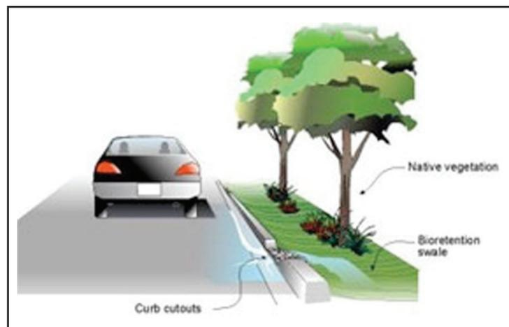
*Figure 2.5a Curb Cuts Schematic*
