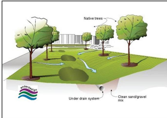
Figure 2.5b Bio-swale Schematic
