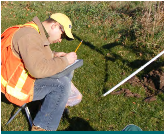
Figure 5.2.2: Fast-moving soils full of gravel and cobble will use a lot of water during testing and augering this material is difficult. Be well equipped with shovels, a sufficient water supply, and other equipment when testing. When soil testing clay materials, bring a comfortable chair. (Source: Aquafor Beech)
