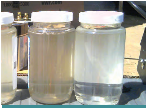
Figure 1.3.1: LID infrastructure performance assessment conducted by CVC and its partners is finding significant gains in water quality with LID. This photograph shows a sample collected from a typical curb-and-gutter road (left) compared to runoff treated by a bioretention LID practice (right). (Source: CVC)
