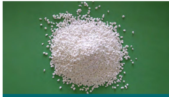
Figure 2.4.6: Engineered media such as phosphorus removal media use a variety of mechanisms to absorb and retain dissolved phosphorus. (Source: Aquafor Beech)
