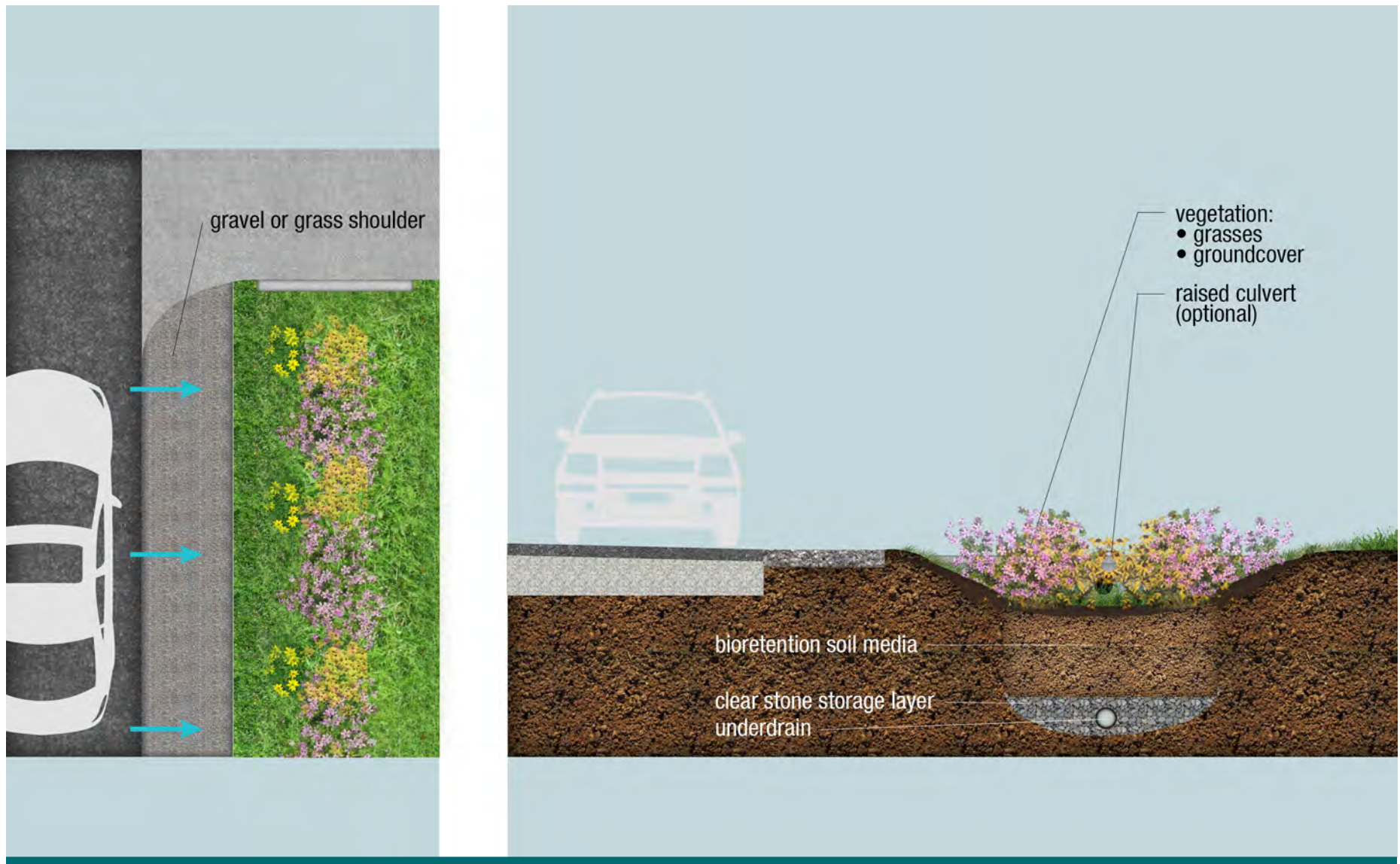
Figure 2.2.5: Bioswale plan view [left] and cross-section [right]
