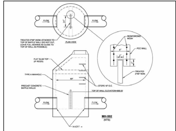
Figure 4 – Water Level Control Structure
