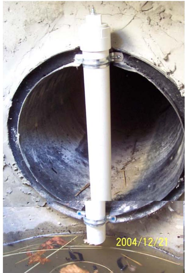
Figure 7 – Water Level Sensor in PVC Housing
