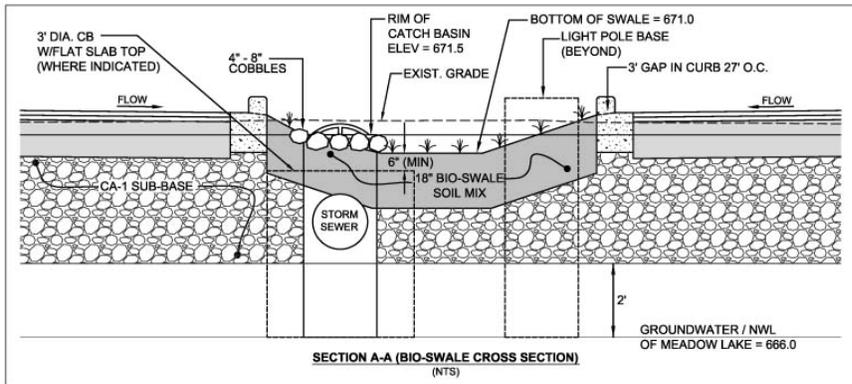
Figure 2 – Bio-swale Cross Section
