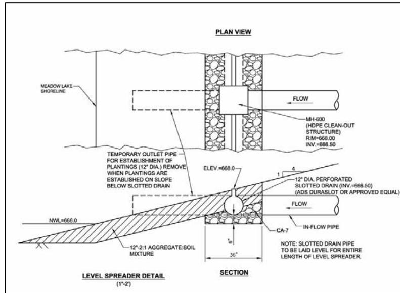
Figure 6 – Level Spreader Detail/Cross Section
