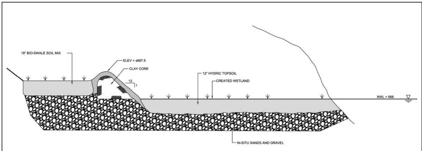
Figure 5 – Created Wetland/Level Spreading Pool Cross Section
