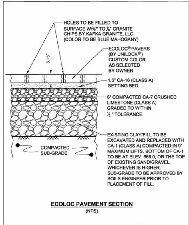
Figure 3 – Permeable Pavement Cross Section
