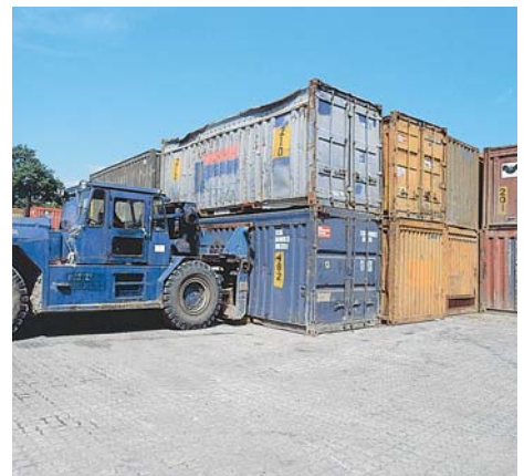
Sterling Sugar container handlers can weigh up to 160,000 lb when fully loaded
