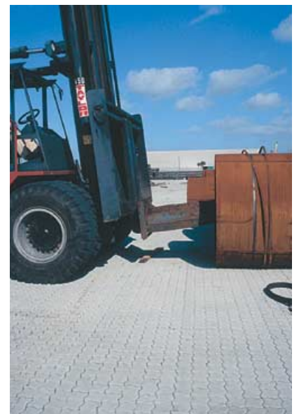
A Taylor TEC-450L transports a roll of coiled sheet steel weighing over 37,000 lb
