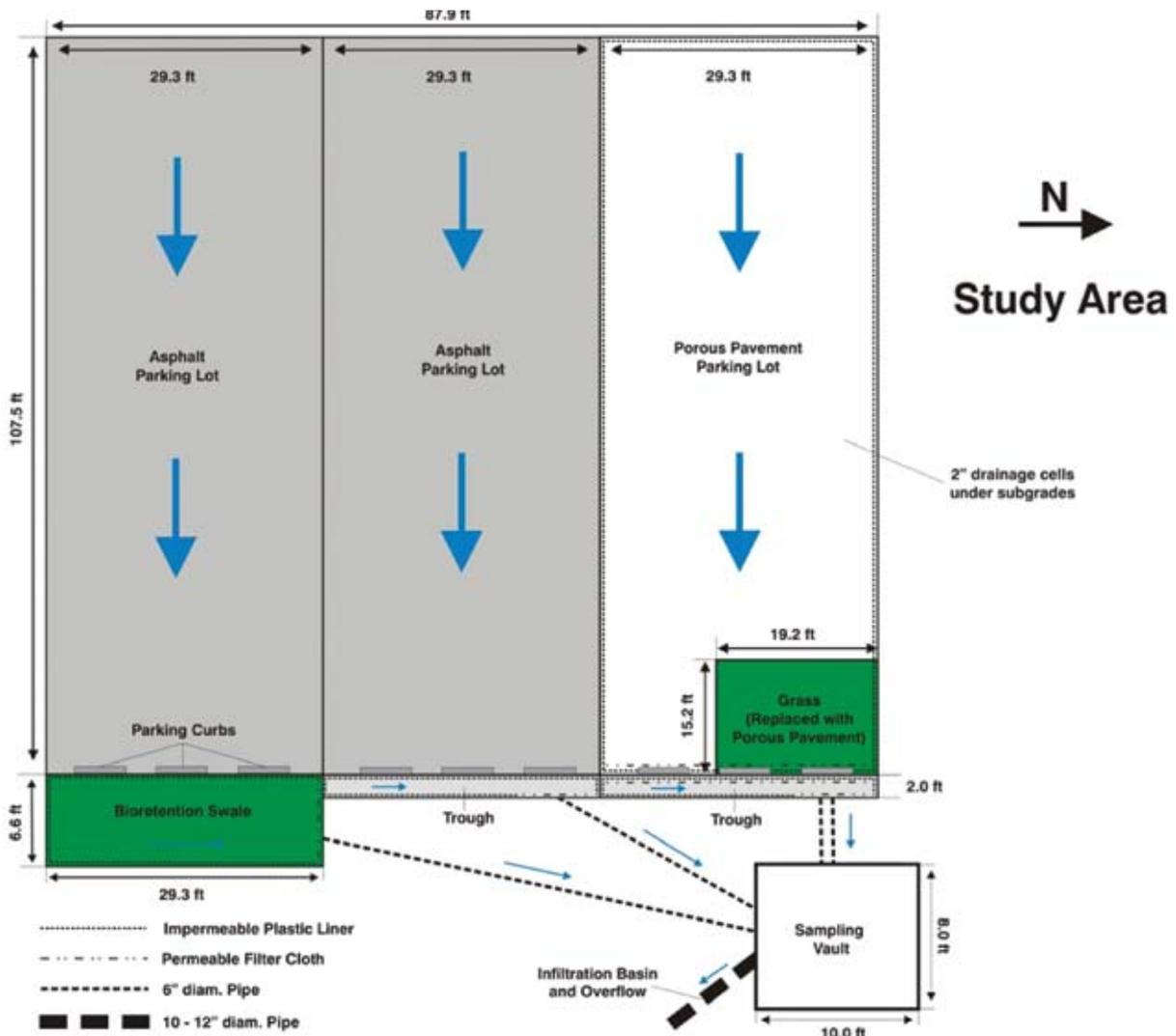
Figure 1. The Seneca College test site evaluates runoff directly from asphalt, from asphalt into a bio-swale as well as surface and subsurface runoff from permeable interlocking concrete pavement.
