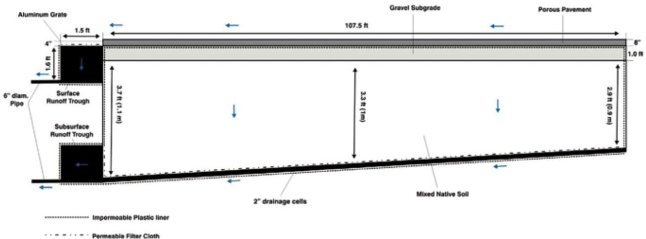
Figure 3. The PICP test area includes subsurface monitoring at the bottom of the open-graded base and further down within the soil subgrade. Water is sampled inside the troughs or utility vaults.
