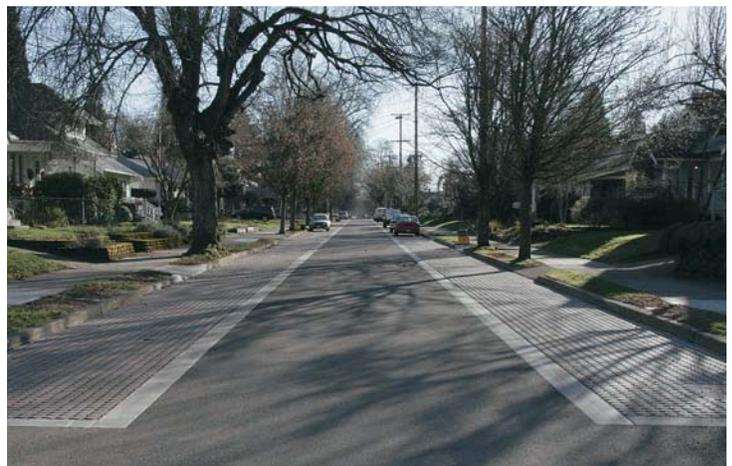
*The center travel asphalt lane slopes towards the permeable Ecoloc® pavers to capture and infiltrate stormwater runoff*
