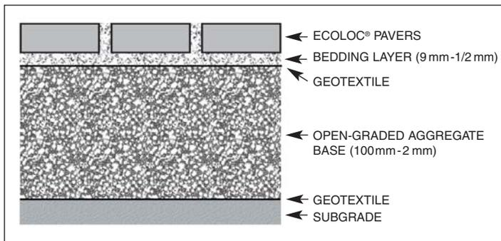
In the pavement cross-sections that utilize the center asphalt travel lane in conjunction with the Ecoloc® parking lanes, the drainage base layer extends
