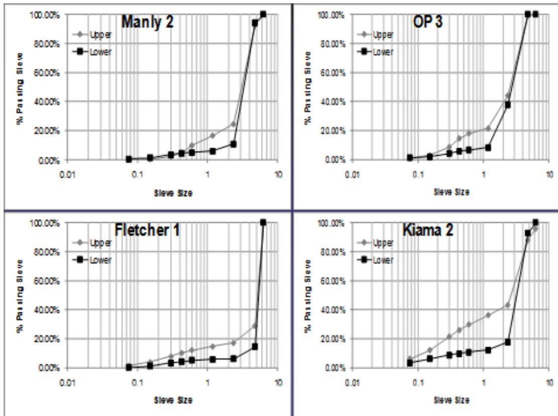
**Figure 3. Typical jointing gradations comparing upper and lower joint material.**
