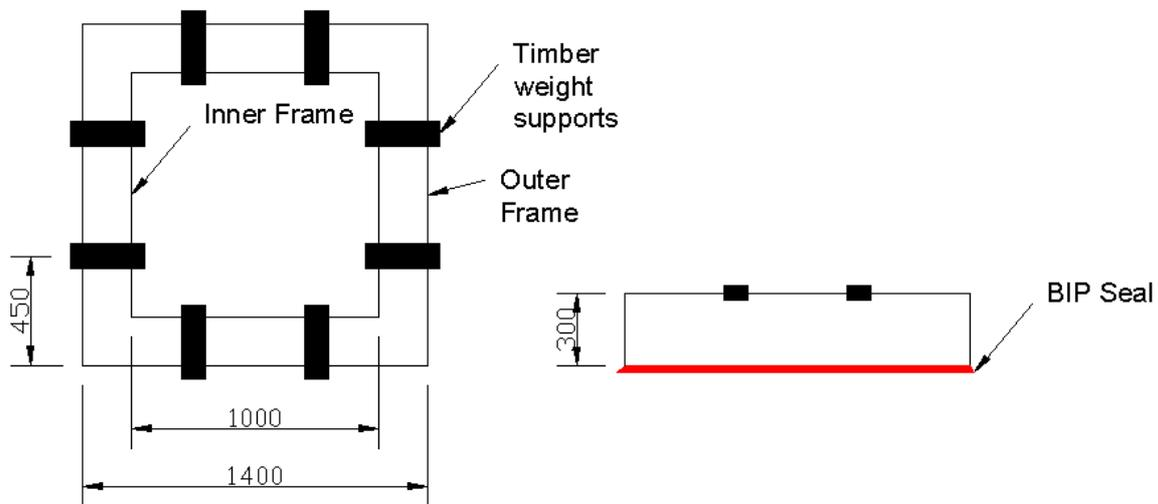
**Figure 1. Double Ring Infiltrometer (all dimensions in mm).**
